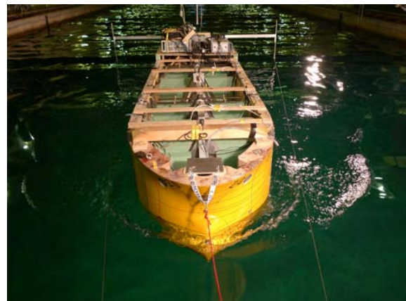
Towed flexible model of an ore carrier.
