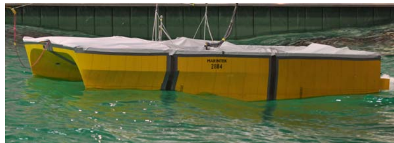
High speed catamaran model with waterjet propulsion.
