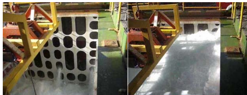
Moonpool water responses are critical for operability of offshore vessels.
