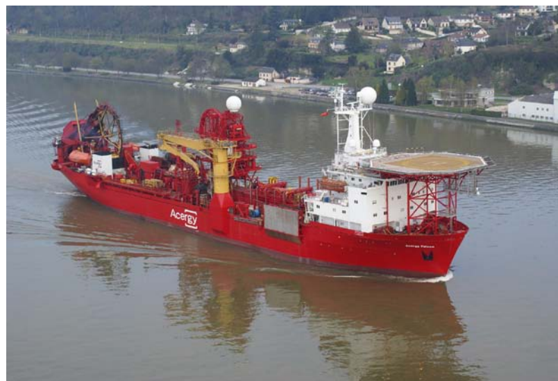
The MEG pipeline installation campaign at Ormen Lange in 2009 was performed by Acergy Falcon.
