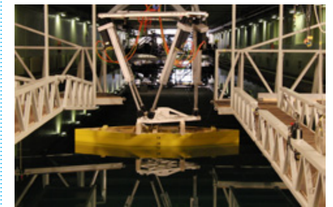
Figure 4. Manoeuvring a model with forced heave motions.
